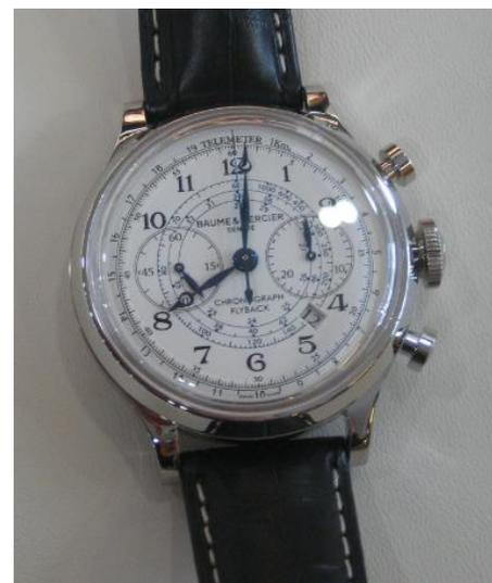
So what is a flyback chronograph you ask? Well it's quite simple, the flyback allows the watch wearer to stop, reset and restart the chronograph function of the watch with the use of one pusher. This allows the wearer to measure short intervals between two events, like two cars crossing a finish line. You simply use the pusher at 2 o'clock to start the seconds hand and then use the pusher at 4 o'clock to reset it and start over, or have the second hand "flyback" to the start.
